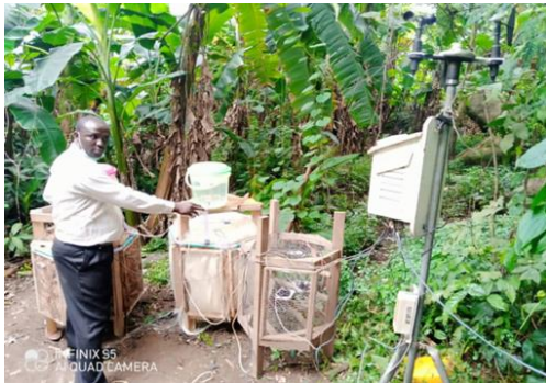
Plate 4. Evaporative cooling structures on site connected to the automatic weather station
