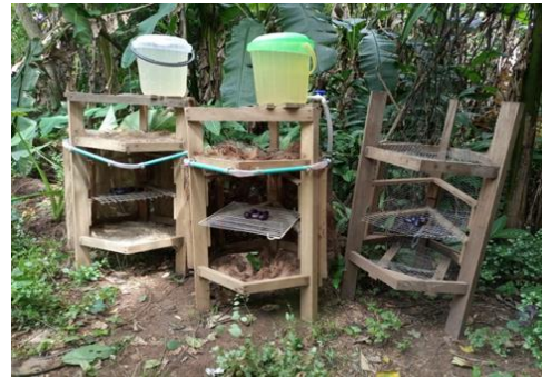
Plate 4. Evaporative cooling structures on site connected to the automatic weather station
